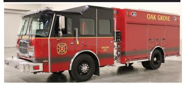
Oak Grove Fire Department recently put into service their new 2014 E-ONE Typhoon eMax Rescue Pumper. This unit is built on a heavy-duty extruded aluminum cab and body. Features include a 178" wheelbase for increased maneuverability, 350hp Cummins ISL9 engine, 1500gpm eMax Pump, 780 gallon tank, FireTech 72" LED Brow Light and Whelen LED scene & warning light package. Sold by Vogelpohl Fire Equipment www.vogelpohlfire.com
