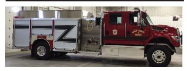
The Boyle County Fire Dept. has taken delivery of a 2015 Toyne Rescue Pumper. This unit is built on an IHC 4400 chassis. It features a bolted stainless steel body, 1500 GPM Hale Pump, 10KW Harrison Hydraulic Generator Set, 1500 gallon tank, and a foam Pro 2002 Class A/B foam system with a 50 gallon foam tank. It also features a remote bumper nozzle for Airport fire/rescue service. The truck was sold by James Riddle - High Tech Rescue, Inc.
