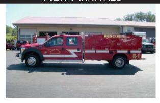
Lincoln Co. FD Station 1: Has taken delivery of a 2011 Wynn Ford F-550 Rescue with an 11' body, 9500# Warn Winch with Receiver Front and Rear, Rear Slide, an EU 3000 Honda Generator, and other miscellaneous equipment.
