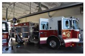
New Toyne Custom Pumper Delivery- Danville Engine 12. This Unit Features a 1500 gpm pump, 500 gal. tank, Akron Foam Induction, 15KW Hydraulic Gen Set built on a Spartan Gladiator Chassis. It was sold by High Tech Rescue, Shelbyville KY.
