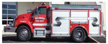
Hillsboro Fire Dept.- Manufactured by Southeast Apparatus, LLC (888-996-6277)...A 2013 Ford F-750 Interface Pumper with a Hale 750-gpm Pump, a 750-gallon poly water tank, and a 12' Rescue Pumper Body.
