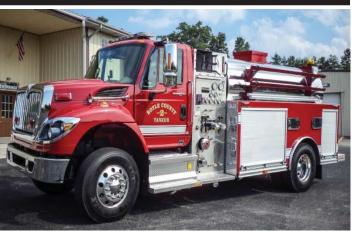
Boyle Co. Fire Dept.- Manufactured by Southeast Apparatus, LLC (888-996-6277)...A 2013 International 7500 Pumper/Tanker with an 1800-gallon tank, a 750-gpm Darley Pump, a powered dump tank rack, and swivel dump valve.
