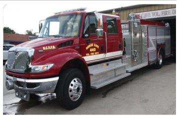
The City Horse Cave VFD has taken delivery of a 2013 Toyne pumper. This unit features an aluminum Body, 1000 Gallon Poly Tank, 1250 GPM Hale QFLO PLUS pump, Foam pro 1600 Class A foam system, and a Honda Genset, built on an International 4400 Crew cab Chassis. The unit was sold by High Tech Rescue Inc.
