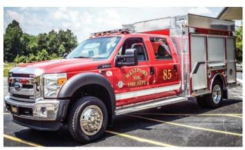
Westport Fire Dept.- Manufactured by Southeast Apparatus, LLC (888-996-6277)...A New 2012 Ford F-550 4x4 Rescue Truck with a 9' Custom 300 Series Aluminum Heavy-Duty Rescue Body, R.O.M. Roll-up Doors, Open Back Design with Line-X Bed Liner, and Skid Unit.
