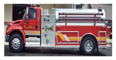
Rural Bradfordsville Fire Dept.- Manufactured by Southeast Apparatus, LLC. (888-996-6277)...A 2013 International 4400 Tanker with a 2000-gal. Polypropylene Stainless Steel Wrapped Elliptical Tank, a Darley 1000-gpm LSP PTO Pump, and a 10" Air Activated Swivel Quick Dump.
