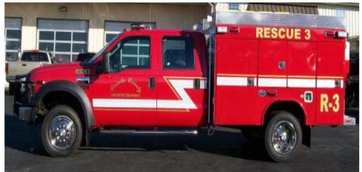
Lincoln Co. Station 3 / Moreland VFD: Has taken deliver of a 2010 Wynn Ford F-550 Rescue, with a 9' open rescue body, a Warn 9500# Winch with full brush guard, a Honda EU3000 Generator, L.E.D. Emergency Lighting, and much more!
