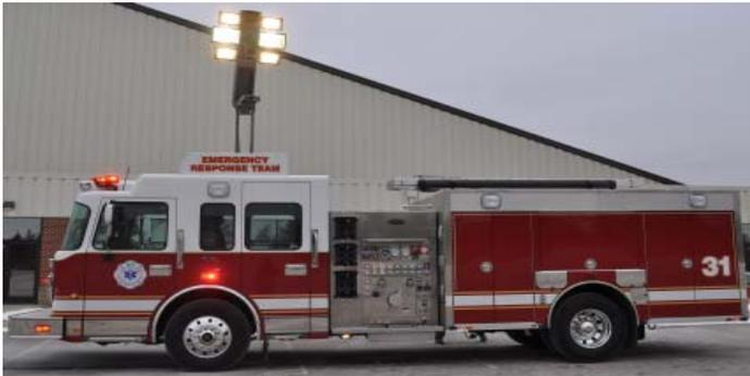
Louisville Gas and Electric Trimble Co. Plant Emergency Response team has taken delivery of a 2010 Toyne Pumper sold by High Tech Rescue in Shelbyville KY. This unit features a Spartan Gladiator Chassis, Stainless Steel Body, Hale Q Pak 1500 gpm Single Stage pump, 750 Gallon Tank, Foam Pro Class A foam system, 10K Gen Set, Remotely operated light tower.
