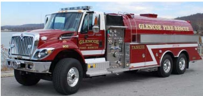
Glencoe KY took delivery of a 3500 Gallon tanker from US Tanker. The unit was sold by High Tech Rescue and features a 3500 Gallon Painted Stainless Poly Tank, Stainless Body, 750 PTO pump, 7500 Series International Chassis.
