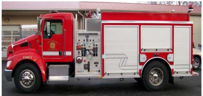
Southeast Floyd FD: Has taken delivery of a 2011 Wynn Kenworth T-370 600 Series Pumper, with a 1000-gallon Polypropylene Tank, a Darley PSM 1250-GPM Pump, On-Spot Tire Chains, a removable Deck Gun, 5200 Watt Generator, and much more!
