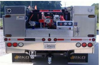
The Masonville Fire Department in Daviess County took delivery of a 2005 F-550 4x4, 4 door cab. It will replace a 1957 brush truck and a 1977 fire/rescue truck. It has 350 gallons of water with a 12 gallon foam tank, 20hp Honda motor, 12,000# winch. It was built by RKO in Madison In.
