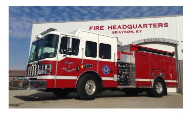
The Grayson Fire Department recently took delivery on new Ferrara Custom Rescue Pumper. The apparatus was purchased from Vehicle Systems. The Chassis is the Ferrara Intruder 2 custom fire chassis; Cummins ISL9 450 hp engine; Allison 3000 EVS transmission; Intruder 2 extended medium cab with 12" raised roof; Seating for 6; 5 SCBA seats with SCBA brackets; Extreme Duty insulation package: 24" extended front bumper with recessed air horns & siren speaker; Polished aluminum wheels
