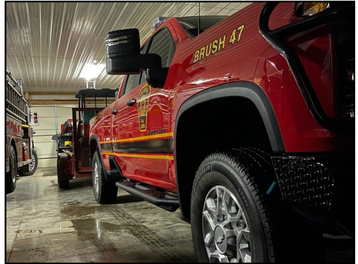
ABOVE: Burna Fire District placed a 2020 3500 Chevy in service with a 250 gallon Enduraplas skid unit with a 10 gallon foam tank from H & R Agra Power of Morganfield. Striping by Rodney Hayes and emergency equipment up fitted by Rapid Response of Paducah.
